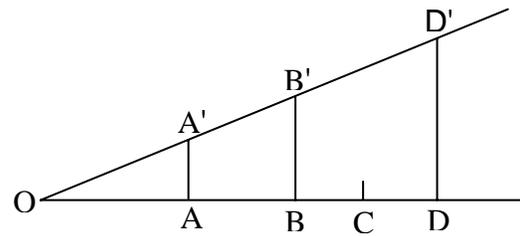
$$\frac{\overline{AA'}}{\overline{OA}} = \frac{\overline{BB'}}{\overline{OB}} = \frac{\overline{DD'}}{\overline{OD}}$$
