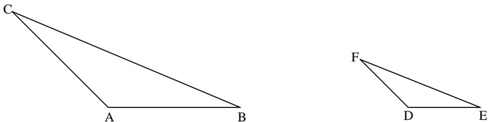
$$\frac{\overline{AB}}{\overline{DE}} = \frac{\overline{BC}}{\overline{EF}} = \frac{\overline{CA}}{\overline{FD}} \Rightarrow \Delta ABC \sim \Delta DEF$$
