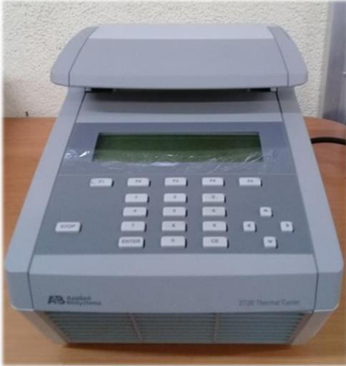
Figura 3. Applied Biosystems 2720 thermal cycler
