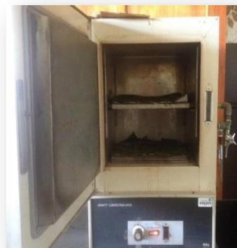
Fig 10: Horno GCA Gravity Convection Oven modelo 2
